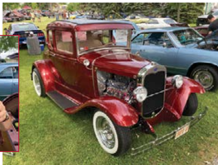
Dave Hirtreiter, of Kenosha, Wis., built this 1930 Ford Model A five-window coupe hot rod. It's powered by a Ford 302-cid V-8 mated to a four-speed manual transmission. Hirtreiter (inset) holds a picture of the "basket case" Model A he purchased in 1982 for $400 and transformed into the immaculate show piece he regularly drives today.
